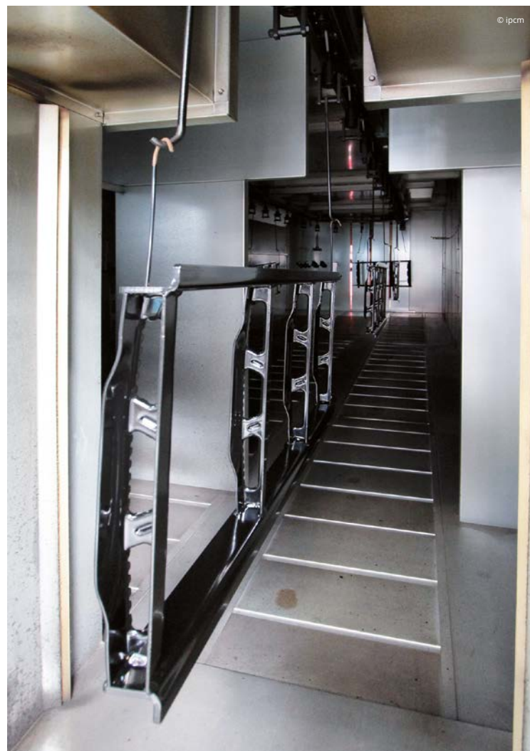
The oven has a single chamber divided into two zones, curing in the first section and drying in the second
