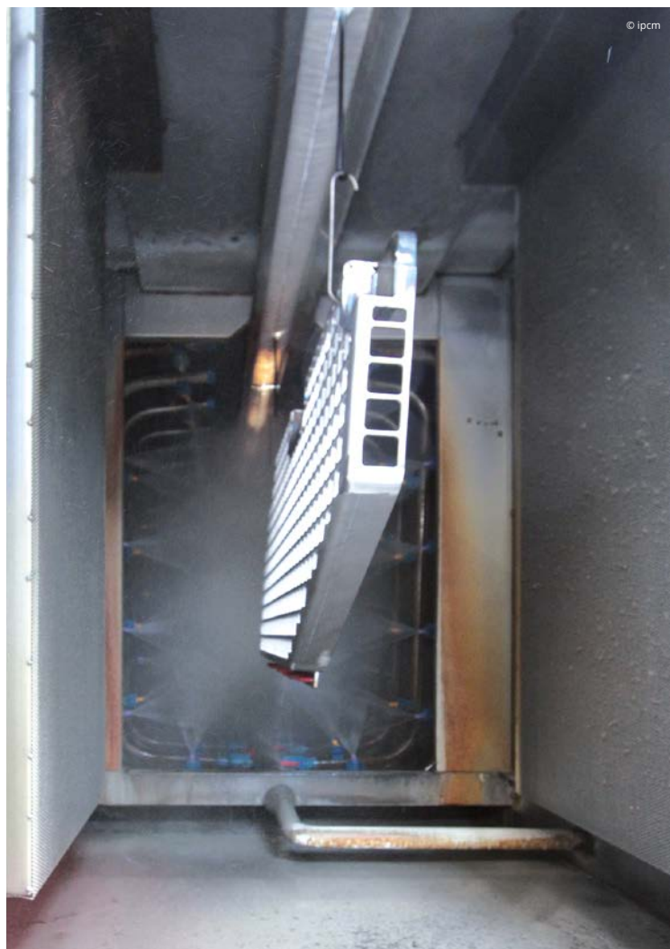
Pieces entering the 3-stages pre-treatment tunnel.
