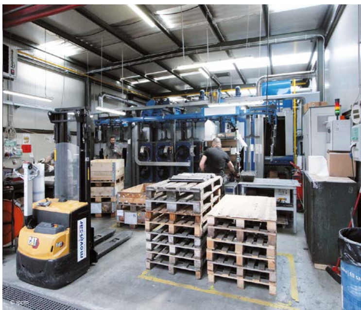
The very compact powder coating line supplied by LEM Impianti.
