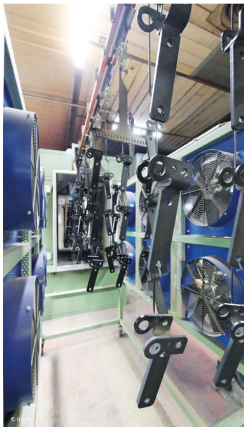
After pre-curing with IR, the parts pass through the cooling zone before entering the booth for the application of the second coat.
