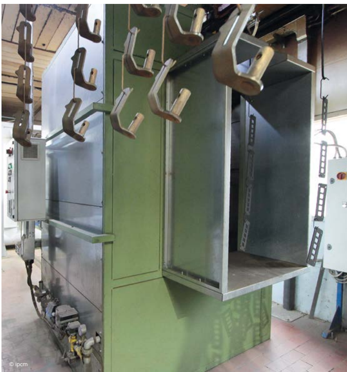
The gelling oven has a length of 150 cm.
